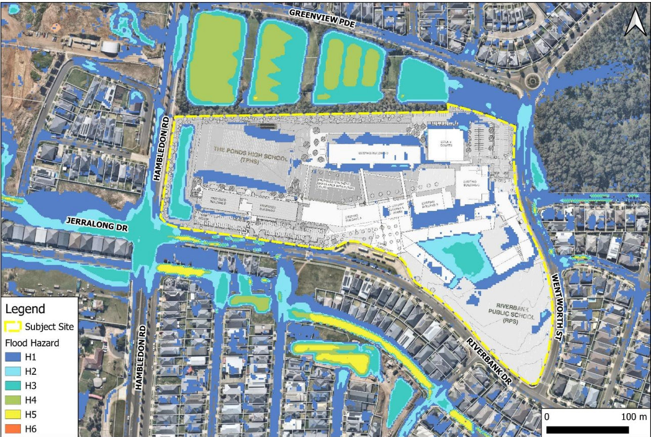
Figure 5: 1% AEP event – flood hazard classification surrounding the site – Post-Development Scenario
