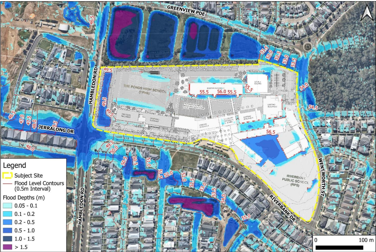
Figure 4: 1% AEP event – flood depths and levels surrounding the site – Post-Development Scenario
